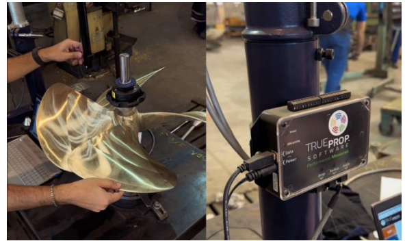
Figure 3: HELIX 48 is a digital pitch measurement system for propellers up to 48 inches in diameter.
