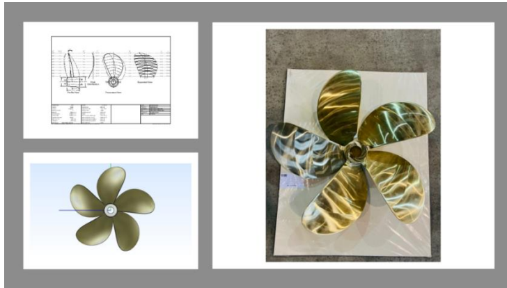
Figure 4: A propeller design for Intermarine shipyard borne from collaboration between HydroComp and Person Hélices.
