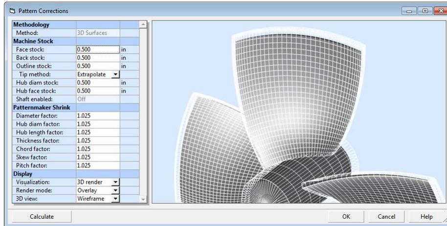
*Pattern Corrections is used to expand and thicken propeller designs to create machining models and casting patterns. Individual control is provided for separate blade parameters.*
