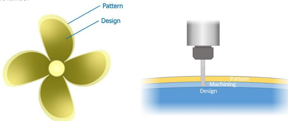
The user is required to specify all machining and shrinkage values for the *Pattern Corrections* utility. This should be done in consultation with the foundry or machining center that is manufacturing the propeller.
