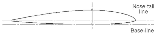
The "base-line" of each section is also known as the pitch line. By viewing all pitch lines from root to tip, a pitch plane is developed.
